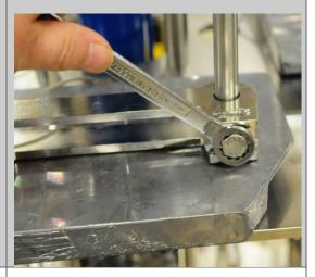
For use in muddy sediment and for better stability, the multi corer comes with 2 footplates. Mount the plates on the lower frame by means of 3 bolts/nuts for each plate.
