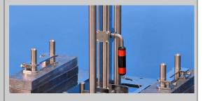
When hoisting the sampler, the sediment tubes are withdrawn from the sediment, and the lids will close to protect the samples from exit.
